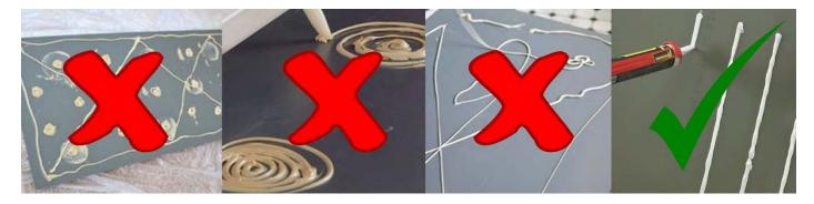
Press the mirror onto the surface being bonded, so that that the adhesive becomes a constant bead thickness of 3mm for optimum cure. Mechanically support the mirror once in place for at least 48 hours. For large mirrors this product should be used in conjunction with mechanical fixings. Within 5 mins of application of adhesive (before surface skin Is formed) the mirror has to be fixed to the wall and positioned in place.
